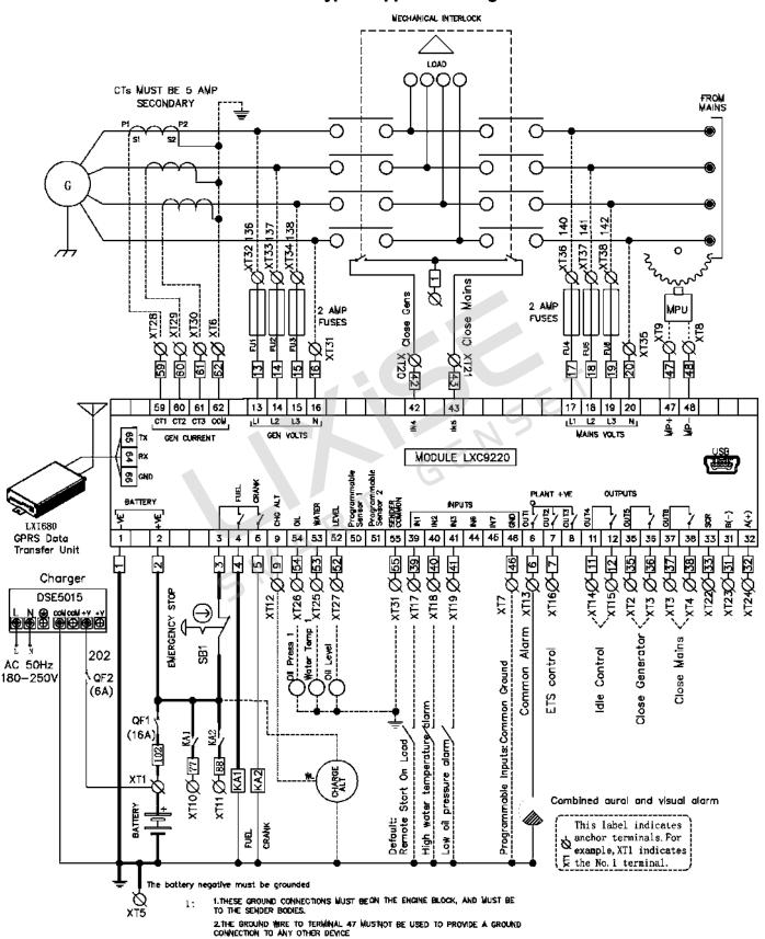
2: 1.The bold solid line indicates 2.5mm2 copper-core wire 2.The bold datted line indicates 1.5mm2 copper-core wire
